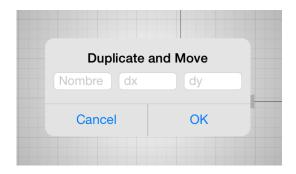
A single new line will be drawn 3-1/2 inches from the bottom. Note that the **new** line is now selected. Tap on the pad to deselect it. Reselect the bottom line, and perform the same action, with the numbers 1 and -29. This gives us the bottom of the center shelf. This time, *leave it selected*, and do it again, 1 and -1. That's the top of our 1 inch thick shelf.
